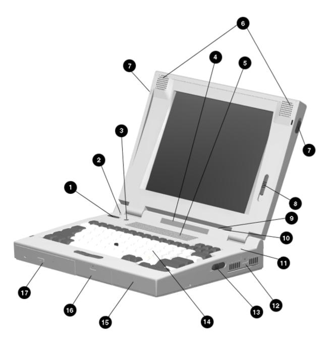
Figure 1-2. Computer Components - Front and Right Sides
